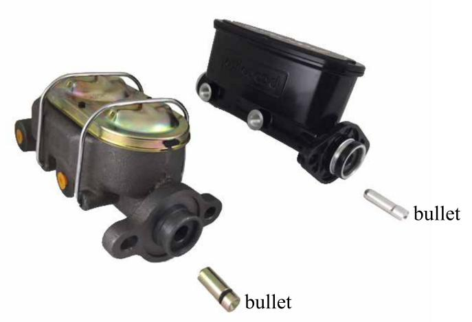
The "bullet" must be installed in the bore of the master cylinder before bolting it up to the hydroboost unit. Without it you will blow up the unit and have to buy another one. Please call if you have any questions.
